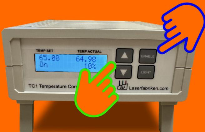
Step 3: Set the temperature using the **Arrow buttons**. Press the up arrow to increase the temperature and the down arrow to decrease it. When you are satisfied with the selected value, click **Enable**. The temperature will then rise steadily, and you can monitor the temperature progress on the screen.
